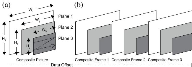
Fig. 1. Principle of planar picture data representation: (a) Still image, (b) video.
